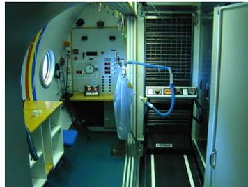
Figures 15 and 16. The Douglas bag system (left) and how it was arranged inside the barometric chamber with the treadmill (right).
